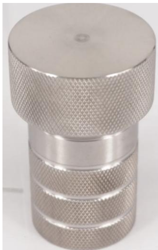
Figure 2.7 A stainless-steel autoclave used for hydrothermal synthesis of zeolites.
