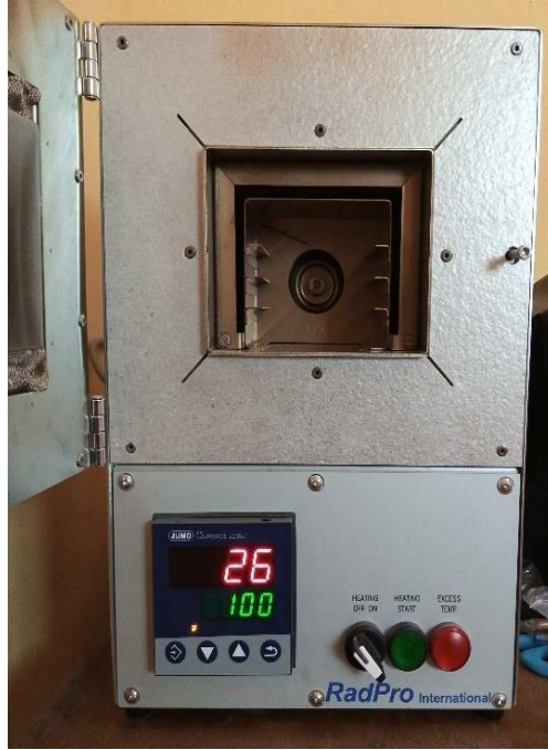
Figure 2.4 A programmable electric annealing oven for pre-irradiation annealing (Esu, 2021)
