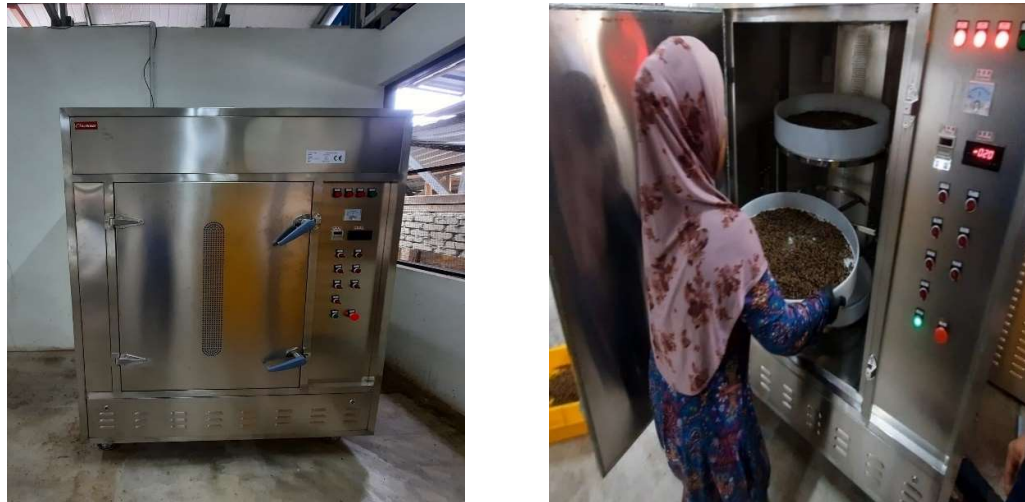
Figure 2.3 Microwave drying of black soldier fly larvae as a part of the Future Animal Feed Innovation Project in Tasek Gelugor, Penang, Malaysia
