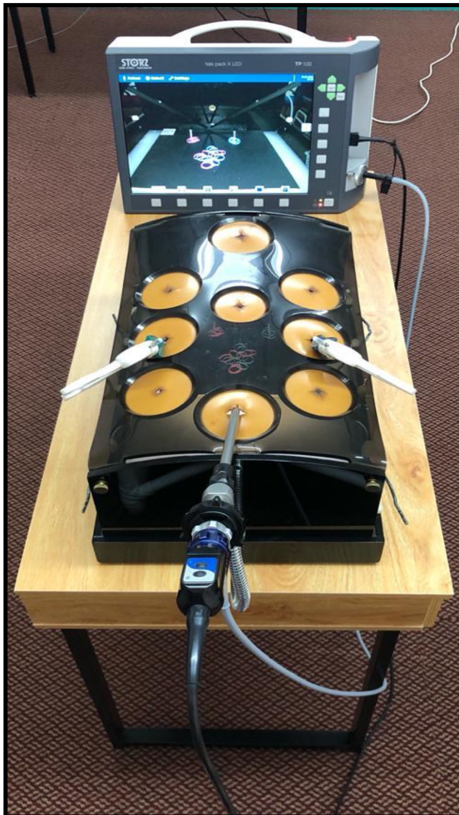
Fig. 8 SZABO-BERCI-SACKIER laparoscopic trainer with endoscope held by flexible endoscope holder and connected to TELE PACK X LED system
