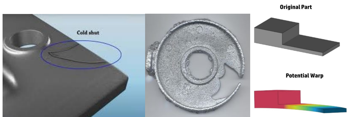
Figure/Rajah 1 : examples of cold shut, misrun and warping in thin casting /contoh tuangan nipis dengan cold shut, misrun dan meleding
