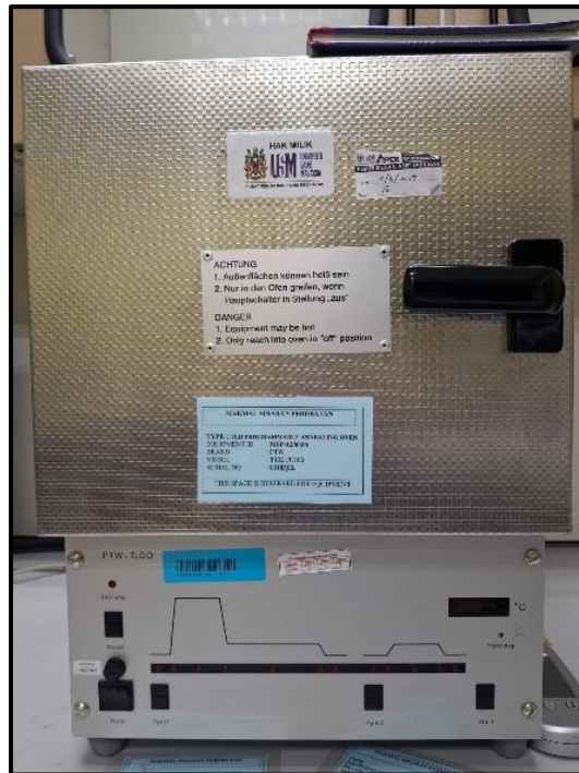
Figure 3.2 The TLD programmable annealing oven at the Medical Radiation Laboratory, PPSK
