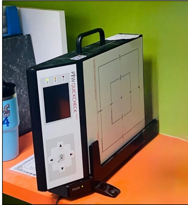
Figure 1.1: PTW QUICKCHECK Phantom placed in its docking station for charging after daily QA use
