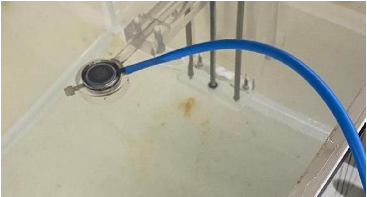
Figure 3.2: Plane-parallel Ionisation Chamber with Model of 34045 Markus®
