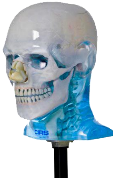
Figure 3.3.1 ATOM Max Dental and Diagnostic Head Phantom Model 711-HN ( PEO Medical, 2015)
