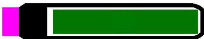
Figure 2-3: The mHDR-v2r consists of a 3.50 mm long cylindrical ^{192}\text{Ir} core with a diameter of 0.60 mm enclosed in a 0.90 mm diameter AISI 316L stainless steel capsule (density 8.06 \text{ g/cm}^3 ) with a small layer of air around the core. The mean photon energy is 360,53 keV [26]
