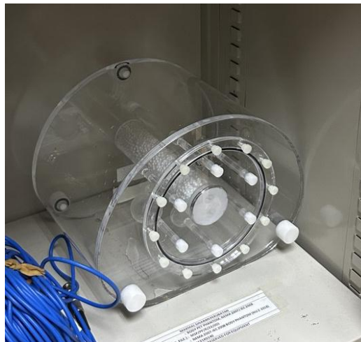
Figure 3.2: NEMA 2007 IEC / 2008 Phantom
