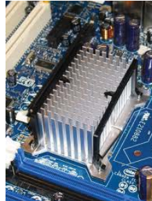
e) Assembly of heat sink on computer CPU board
