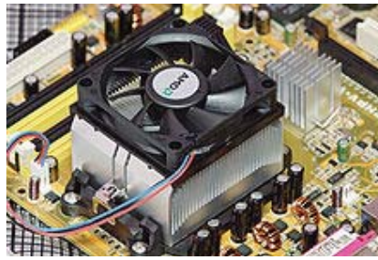
Figure 1.1: Computer processor cooling by heat sink with the application of fan.
