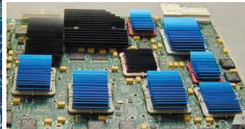
e) Assembly of heat sink on computer CPU board
