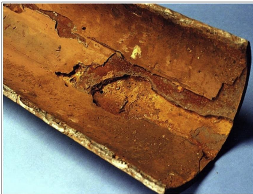
Figure 2.2: Internal corrosion of a crude oil pipeline (Askari et al., 2019).
