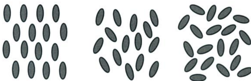
Figure 2.1 Illustration on molecular arrangements of a solid (left), liquid crystal (middle) and isotropic liquid (right) (Silbey, 1987).
