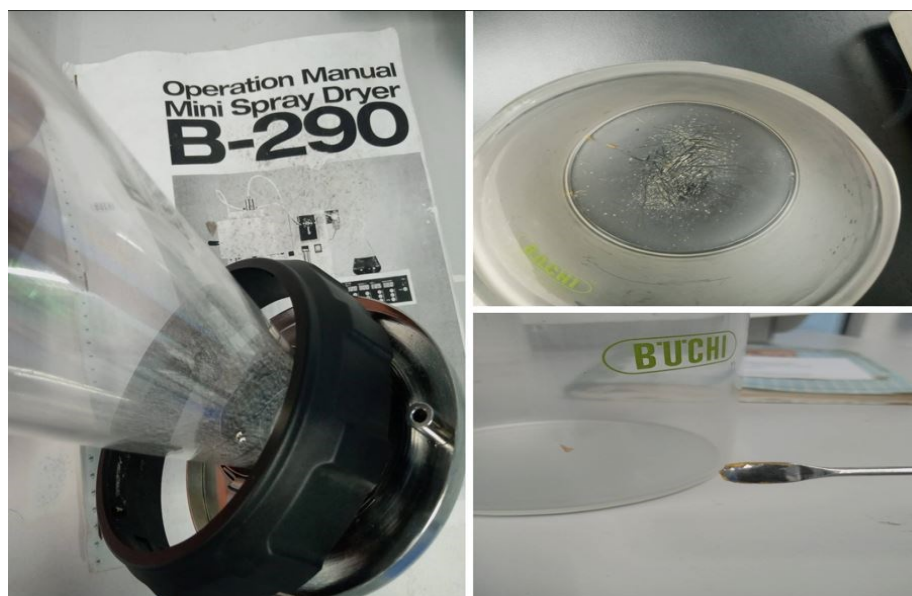
Figure 4.5 LRP exhibiting adhesive properties, adhering to the walls of the spray dryer cyclone and even the collection vessel.
