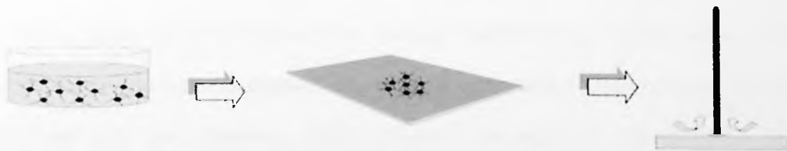
Figure 2.14: The schematic of growing ZnO nanostructure on the substrate (Hung and Whang, 2003).
