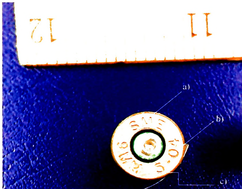
Figure 4.1: Cartridge base. a) Manufacturer; b) Batch number; c) Caliber of cartridge.
