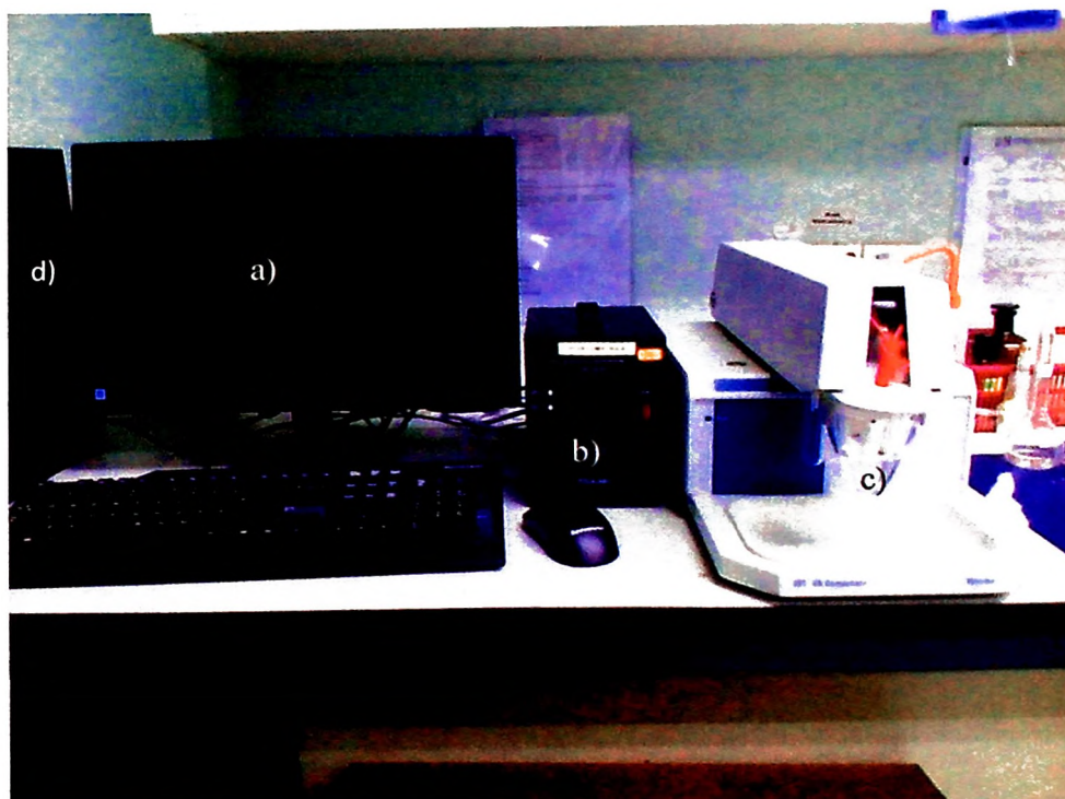
Figure 4.5: 797 VA Computrace. a) monitor; b) voltage supply; c) voltammetric cell d) CPU.
