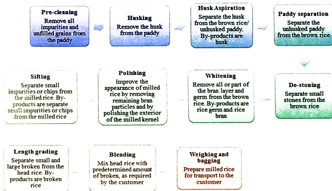
Figure 2.3: The rice milling process (Adapted from International Rice Research Institute (IRRI), 2009).
