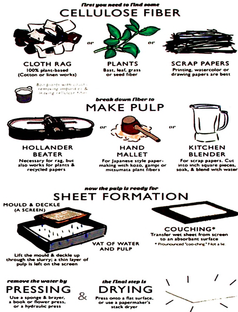
Figure 2.1 The process of paper making (www.paperslurry.com accessed on June, 17, 2016)
