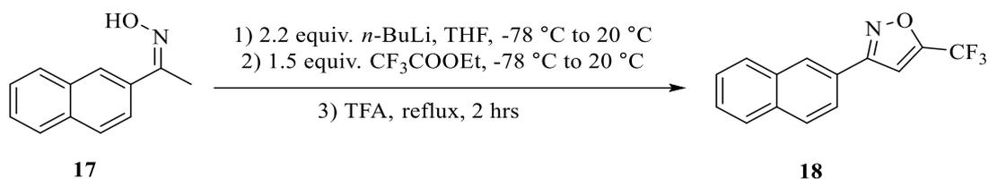
Scheme 2.3 Synthesis of 3-(naphthalen-2-yl)-5-(trifluoromethyl)isoxazole (**18**).
