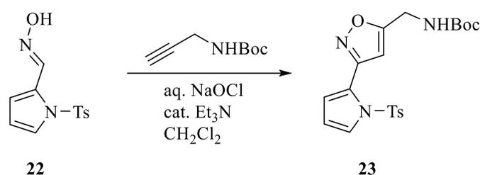
Scheme 2.5 Synthesis of *tert*-butyl ((3-(1-tosyl-1*H*-pyrrol-2-yl)isoxazol-5-yl)methyl)carbamate (**23**) *via* cycloaddition reaction.
