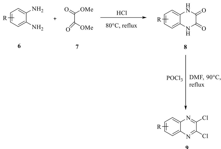
Scheme 2.2 Synthesis route of 2,3-dichloroquinoxaline derivatives.
