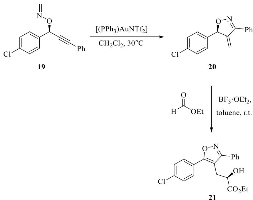
Scheme 2.4 Synthesis of ethyl (*R*)-3-(5-(4-chlorophenyl)-3-phenylisoxazol-4-yl)-2-hydroxypropanoate (**21**) via cycloisomerization reaction.
