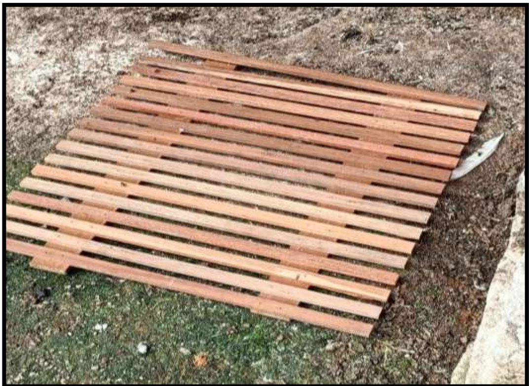
Plate 2.9 Scudder grill used as tool to calculate the fly index at farms
