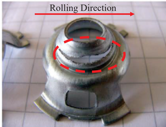
Figure 1: Photograph of fracture of steel 2. The fracture in direction of rolling of material shows worse workability of sheet in transversal direction
