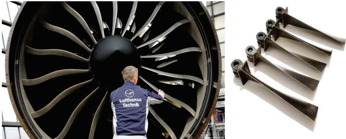
Figure 1 Aerospace engine titanium alloy fan blades
