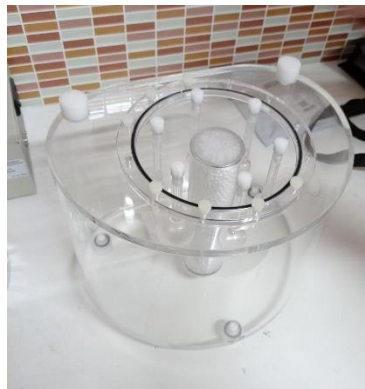
Figure 3.2: NEMA 2012/IEC 2008 phantom
