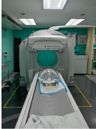
Figure 3.6: The arrangement of the phantom for image acquisition
