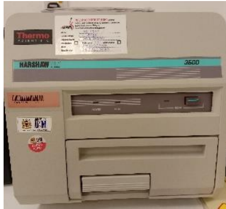
Figure 3. 4. Harshaw model 3500 manual TLD reader (AMDI)
