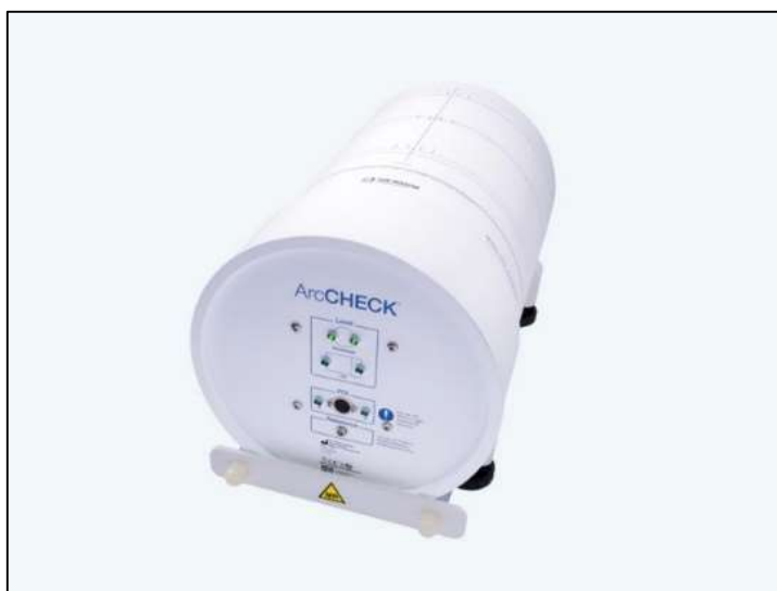
Figure 2.10: ArcCHECK phantom (Sun Nuclear Corporation, n.d.).
