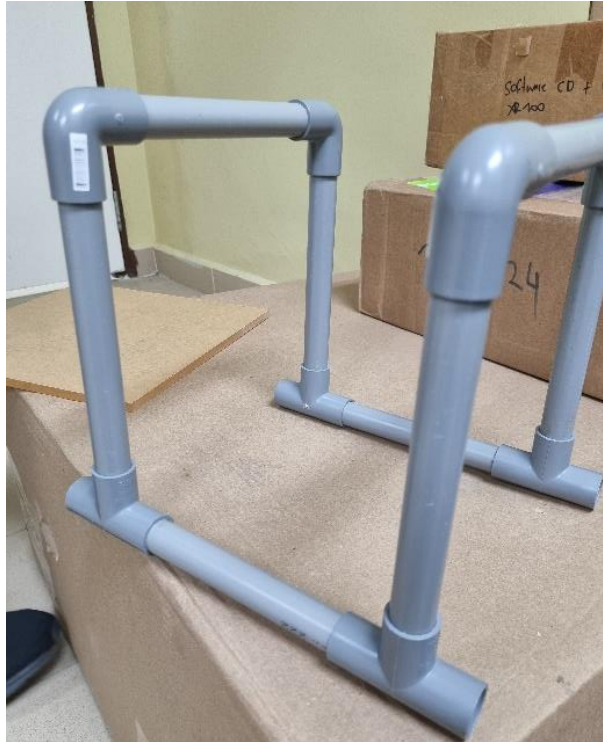
Figure 3.8 Fabricated stand used to place the phantoms during irradiation.
