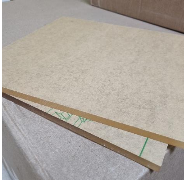
Figure 3.7 Perspex® slabs phantom used to determine mass attenuation coefficient.
