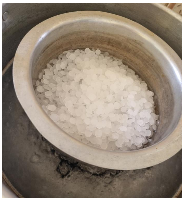
Figure 3.10 The Paraffin wax was melted in double boiling method
