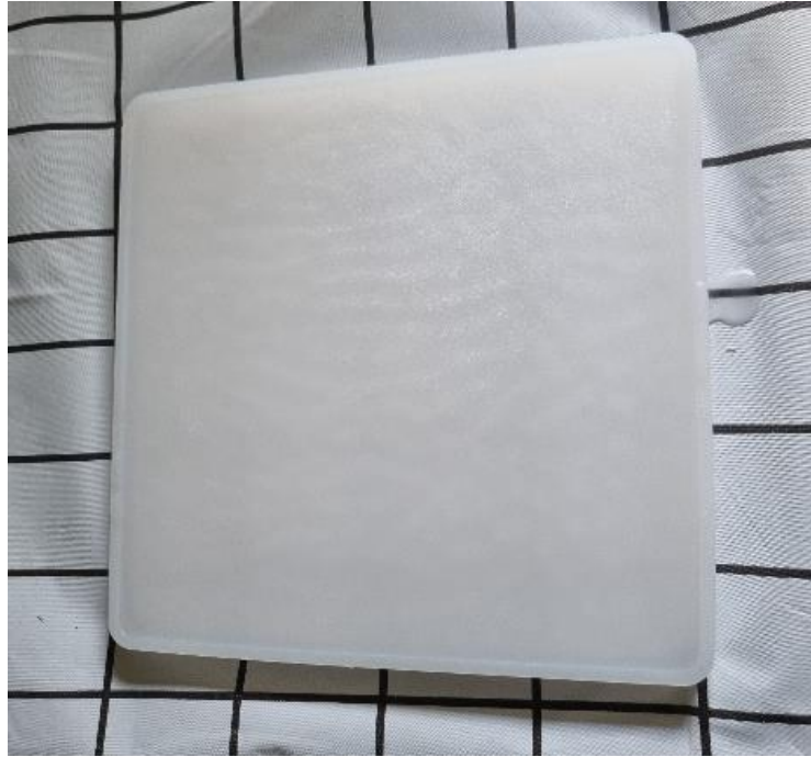
Figure 3.11 The melted paraffin wax was poured into a silicon mould.
