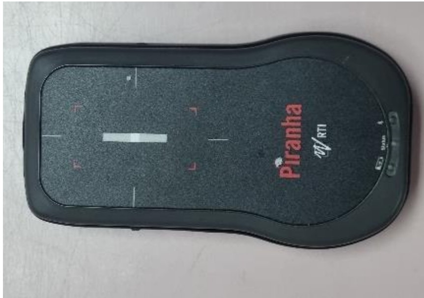
Figure 3.2 RTI Piranha Meter to measure the radiation output of the x-ray beams.
