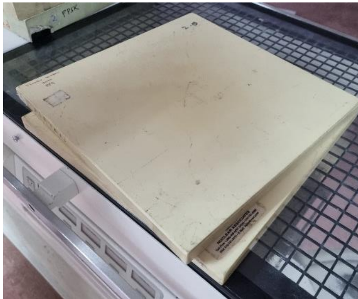
Figure 3.6 Solid water phantom used to determine mass attenuation coefficient.
