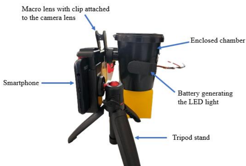
Figure 3.2 The design of the smartphone accessory used during the experiment
