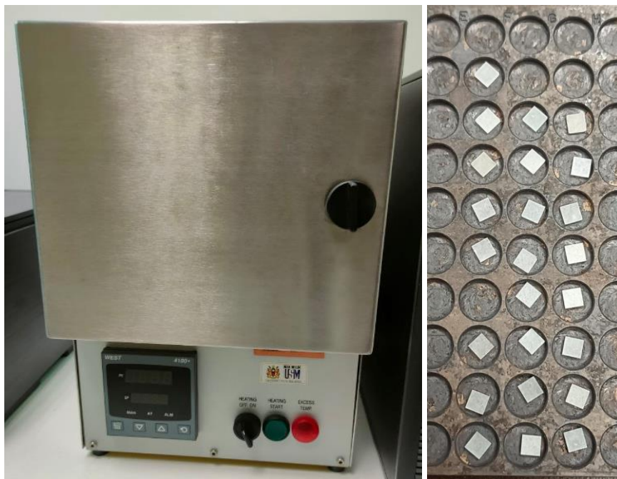
Figure 3.1 of TLD annealing oven (left) and the TLD inside the annealing plate (right)
