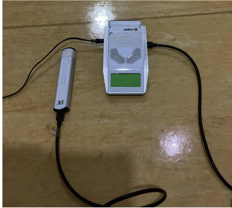
Figure 3.2 The figure shows the solid-state detector (Raysafe, Unfors Xi)
