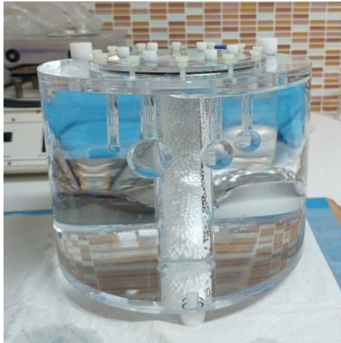
Figure 3.2: NEMA 2012/ IEC 2008 phantom.
