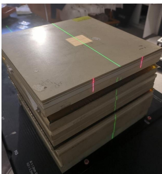
Figure 3.16: OSL measurements in the presence of metal plates
