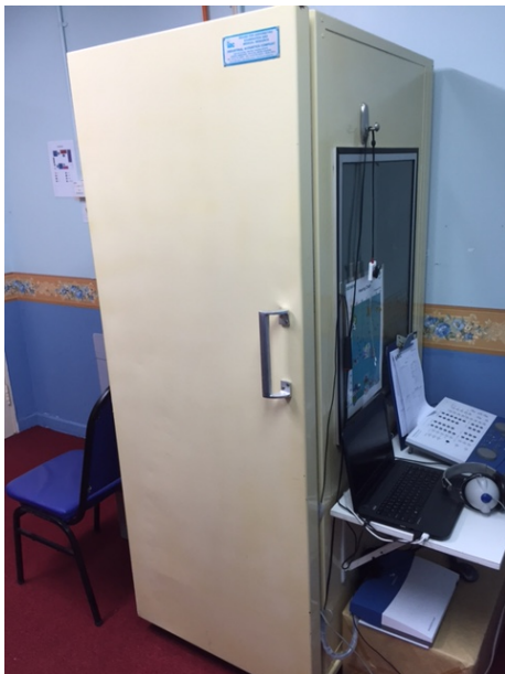
Figure 4.1 Sound proofcabin by Industrial Acoustic Company model 800a (from the United Kingdom) which was placed in a sound-treated room.
