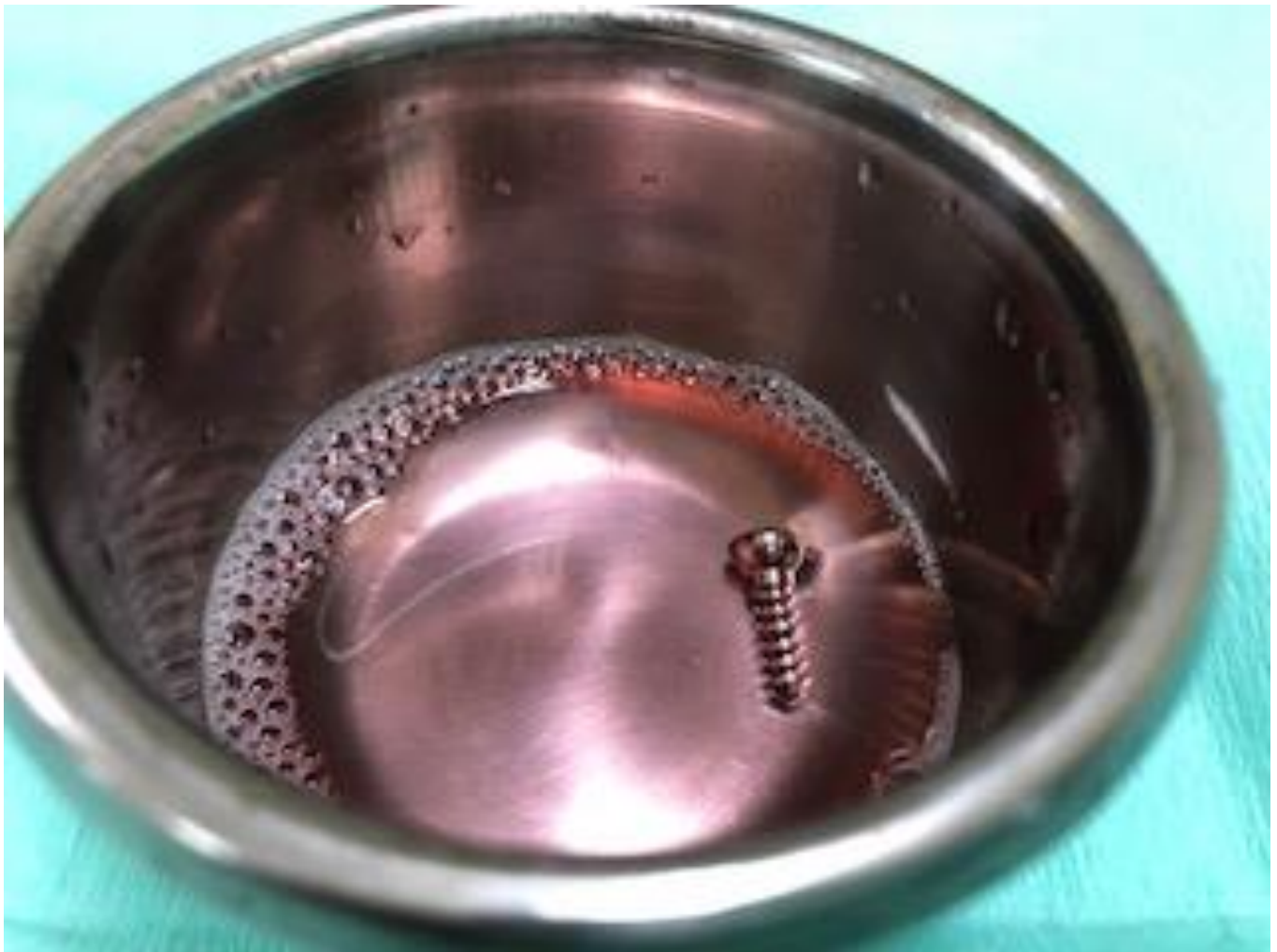
Picture 1: 20 cc of solution was required to fully submerge the 3.5 x 16 mm screw
