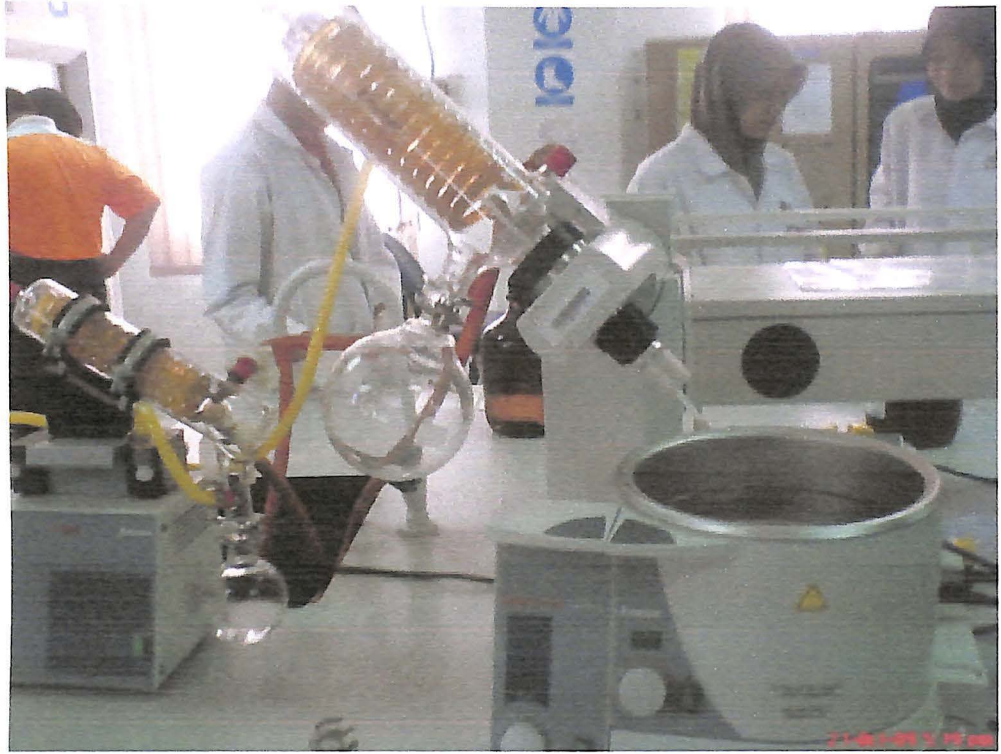
Figure 4: Rotary evaporator used to concentrate the extracts
