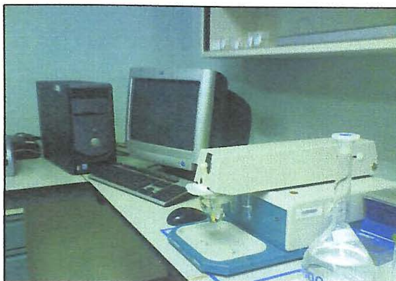
Figure 4.1 Metrohm 757 VA Computerace Voltammetric Analyser combined with Multimode Electrode (MME) System
