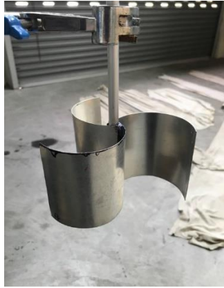
Figure 3.2: Simple model of savonius turbine
