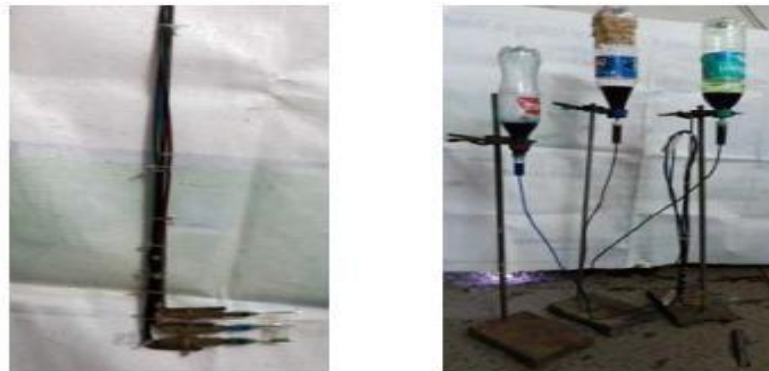
Figure 2.1: Syringe needle(left), dye injection system (right) (Kalyankar et al., 2015).
