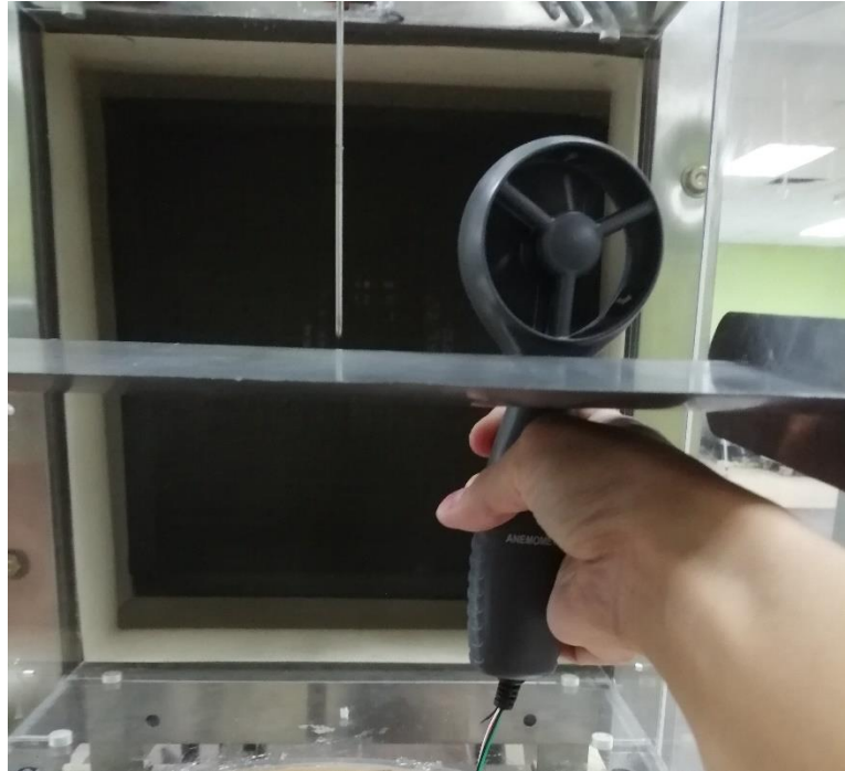
Figure 3. 11: Using a digital anemometer to measure the air speed of wind tunnel
