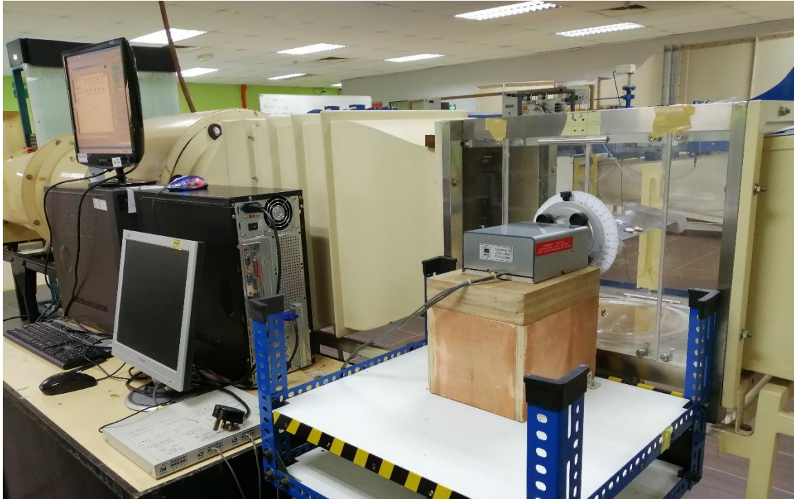
Figure 3. 7: Overall setup of DAQ Electronic Balance in recording the data
