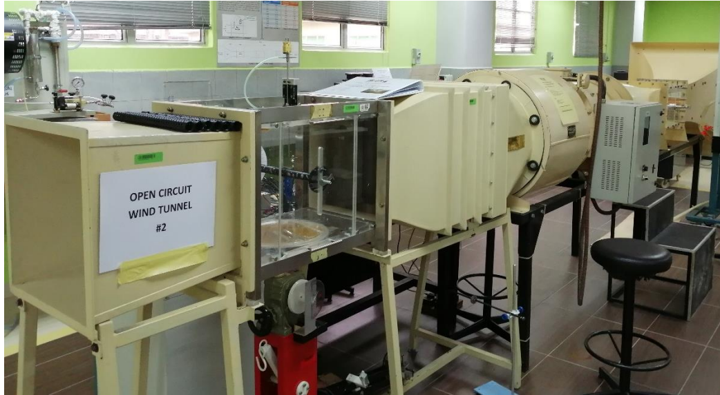
Figure 3. 3: Set-up of open-circuit wind tunnel with bi-test-section
