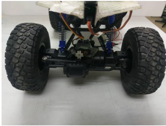
(a) Servo and wheels not actuated
