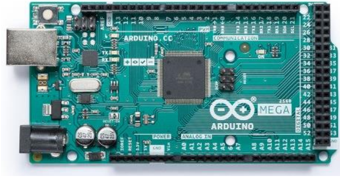
Figure 3. 2: Arduino Mega 2560 board (image courtesy of Arduino.cc)
