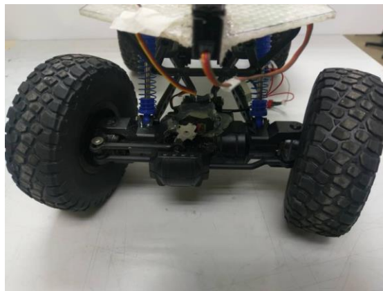
(b) Servo and wheels actuated to the right
