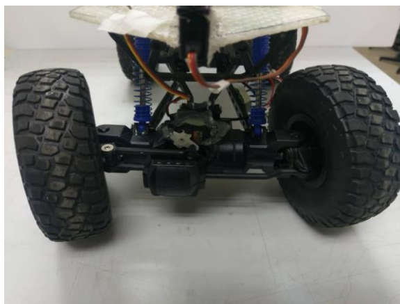
(c) Servo and wheels actuated to the left
