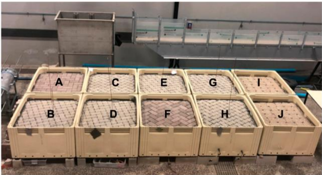
Figure 2.1: PICP Test Cells (Cell A and Cell F laid with Aquaflo® pavers, Cell B, C, D, E, G, H laid with Permealock® pavers, and Cell I and Cell J laid with ‘traditional’ exposed pavers) (B. K. Liu and Armitage, 2020)
