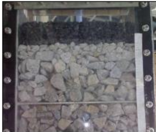
Figure 2.6: Assembly of Porous Asphalt Slab Inside Water Flow Simulator's Body (Hamzah et al., 2013)
