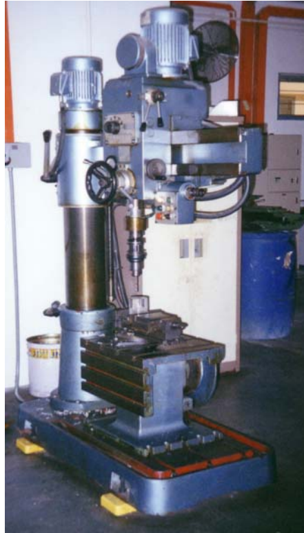
Figure 3.3 The hydraulic drilling machine used to make holes
