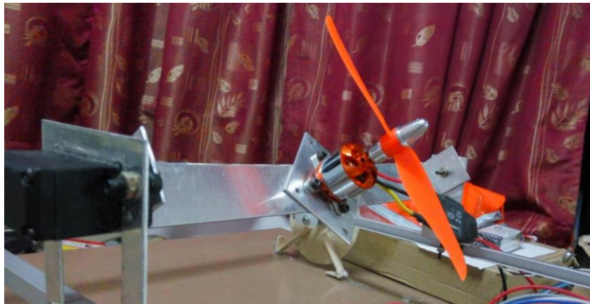
Figure 3.4: Pushing mechanism by using propeller in wall climbing robot.
