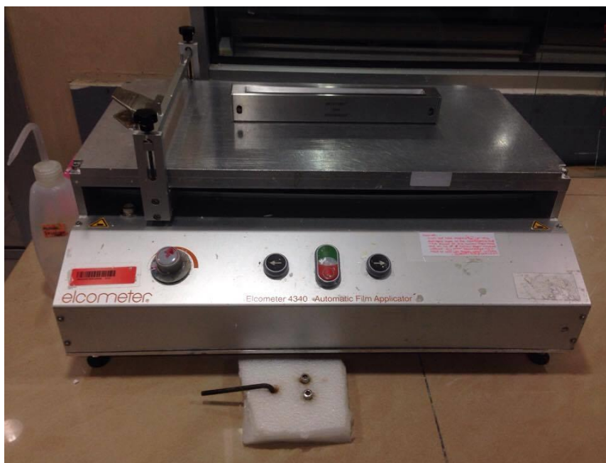
Figure 3.3 Casting machine (Elcometer 4340 automatic)
