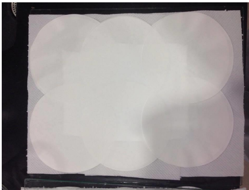
Figure 3.6 Wet membrane then was dried in ambient temperature.
