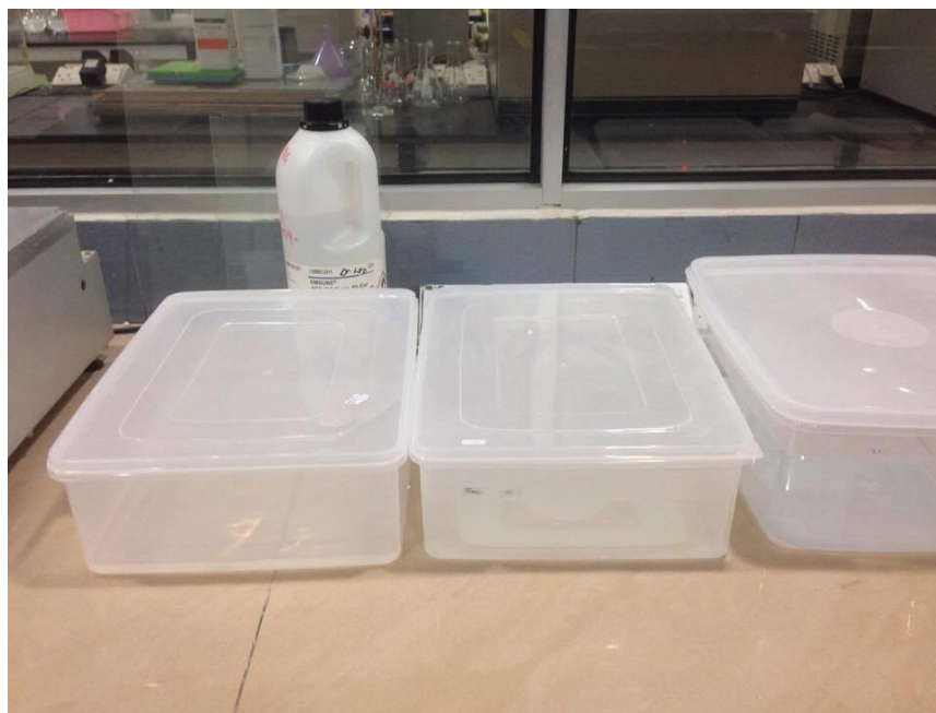
Figure 3.5 The cast film was immersed into the first and second coagulant bath.
