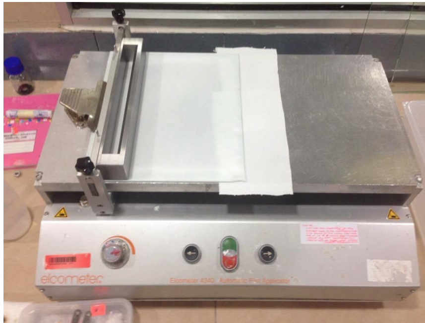
Figure 3.4 Cast film ready for casting process (Elcometer 4340 automatic).
