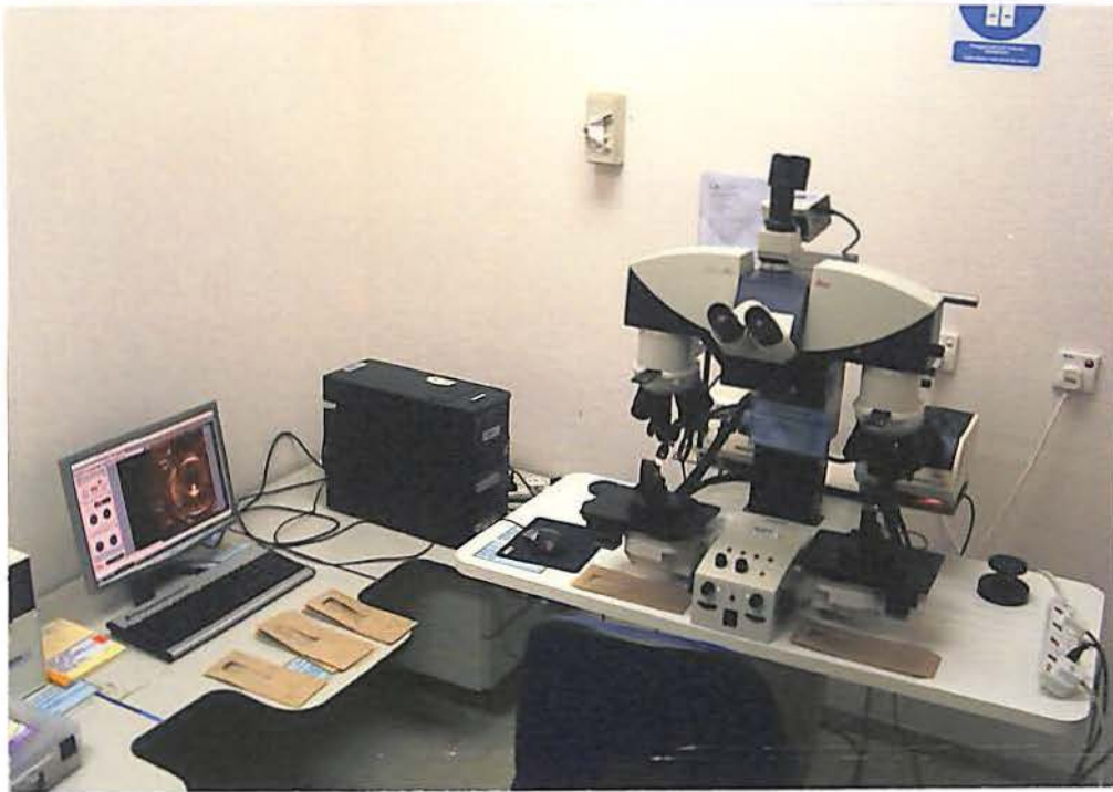
Figure 2: Leica FS C (Forensic Solution Comparison) Microscope integrated with Cold Light Source KL 2500 LCD fiber optic illumination, Leica DFC 290 digital camera and Leica Application Software (LAS).
