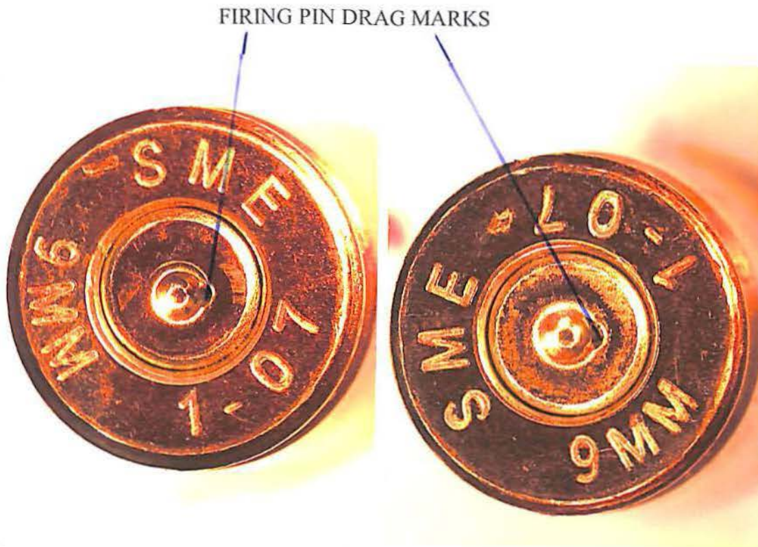
Figure 3: Firing pin impression produced by AS model (left) and QA model (right).
