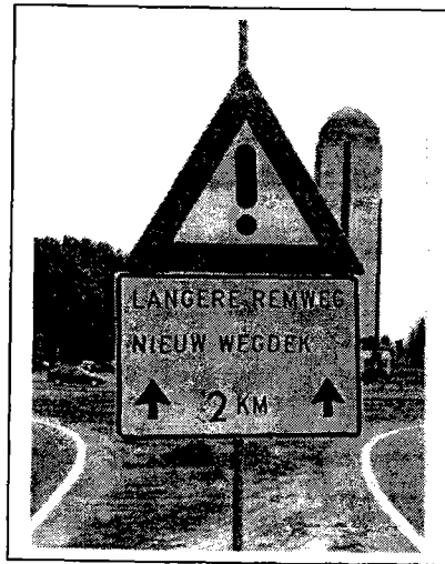
Figure 3 An Example of a Warning Sign on Newly Paved PA Surfacing (Source: DWW)
