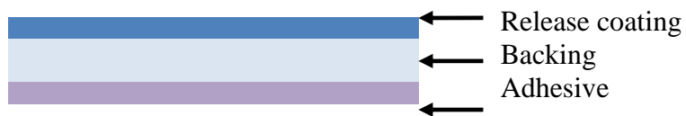
Figure 2.1: Typical construction of Pressure-Sensitive Adhesive
