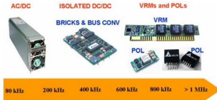
Figure 1.2: Switching frequency of different voltage regulators [1]
