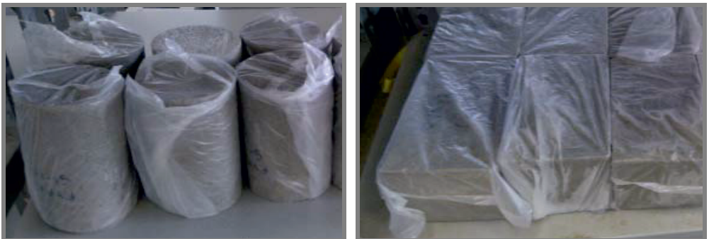
Figure 2. Samples wrapped in plastic sheet for curing
