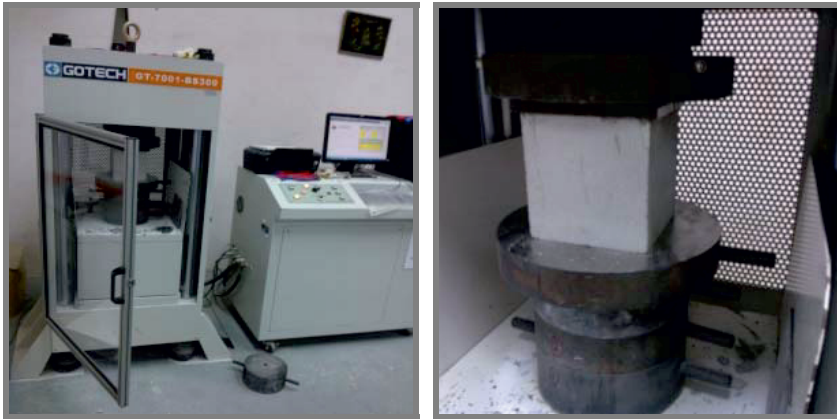
Figure 3. GOTECH GT-7001-BS300, with a 300ton-capacity compression machine.
