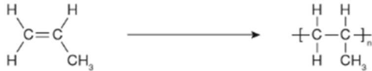
Figure2.3: Polymerisation of propylene to form polymer of polypropylene (Doran and Cather, 2013).
