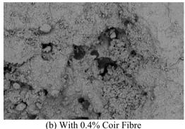
**Figure 1.** Comparison of pore formation between normal foamed concrete (control) and foamed concrete with different percentages of coir at 1350 kg/m<sup>3</sup> density
