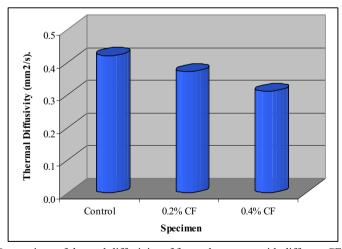
Figure 4. Comparison of thermal diffusivity of foamed concrete with different CF percentages
