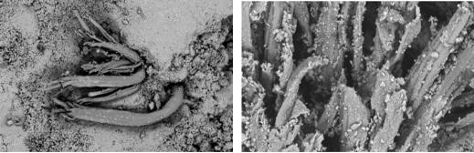
Figure 2. Components of coir fibres which can be seen in the cement matrix
